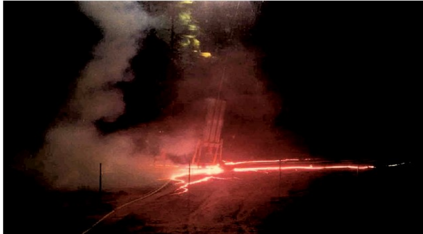
Figure 5 Surface arcing during a rocket-triggered flash; lightning channel outside the field of view [adapted from Fisher et. al. 1994 ( http://www.rakov.ece.ufl.edu/teaching/5490/Effects&LPS_Section%209.pdf )]
